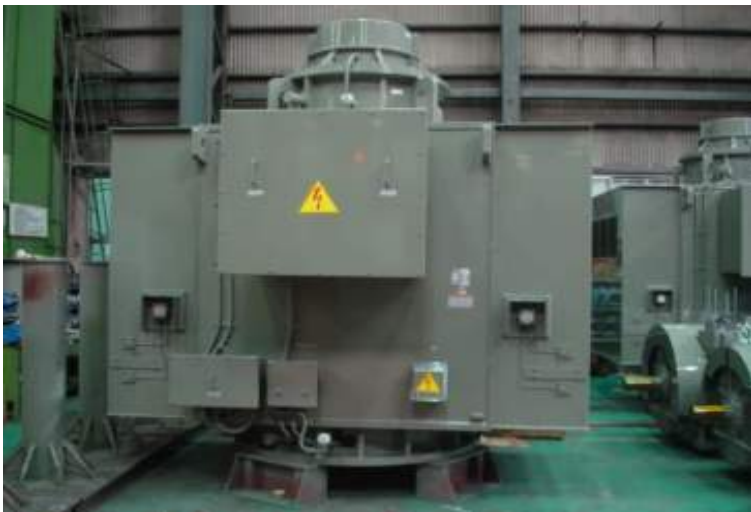
2,500HP 18P 4.16kV 60Hz WP11 VSS Motors for Pump Station
