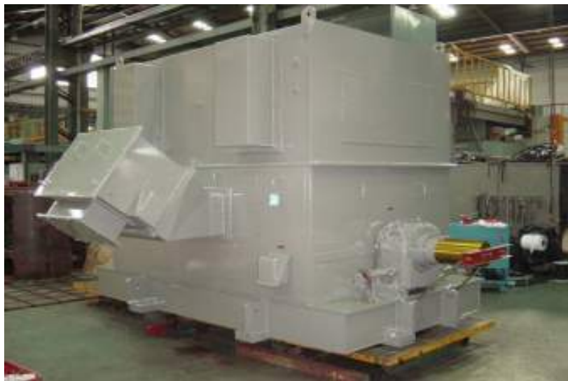
8,840 kW 4P 6.6kV 60Hz TEWAC Motor
