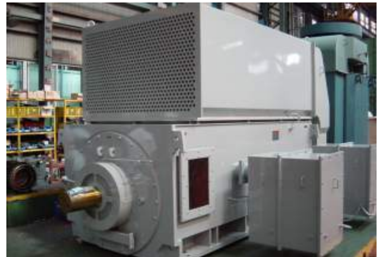
2,800kW 6P 6kV 50Hz TEAAC Wound Rotor Motor for Cement Mill(Exported to Vietnam)
