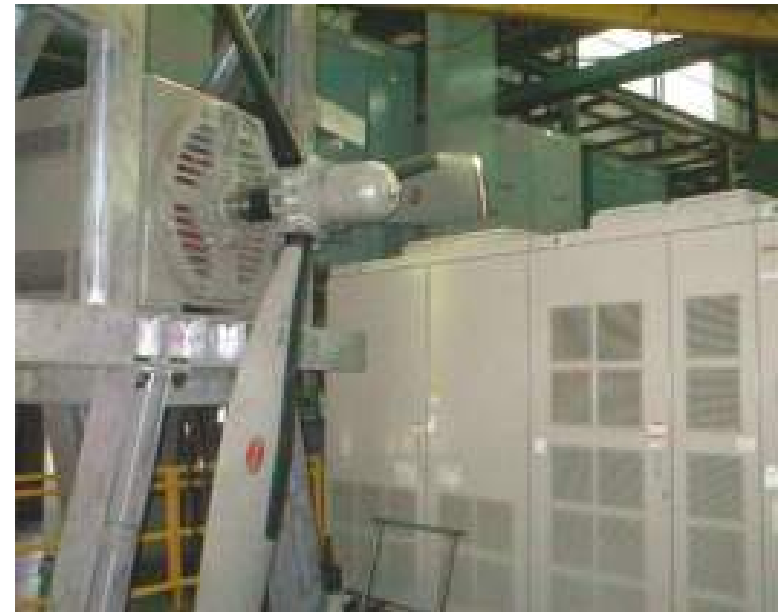
1,500 kW 4P 3.3kV 80Hz ODP Inverter Drive Motor for Wind Tunnel Fan
