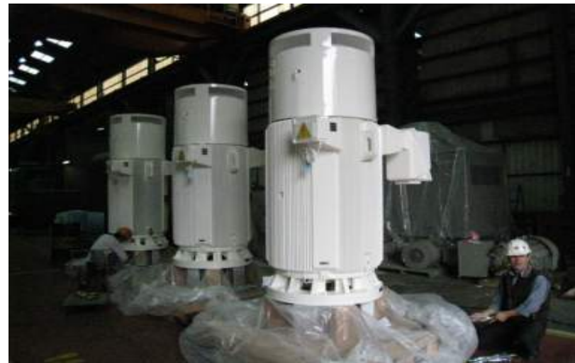
1,250 HP 4P 2.3\4.16kV 60Hz FIN TYPE VSS High Thrust Motors for Water Pumps
