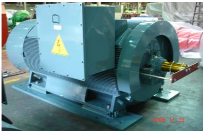
2500HP 6P 4kV 60Hz TEFC Motor
